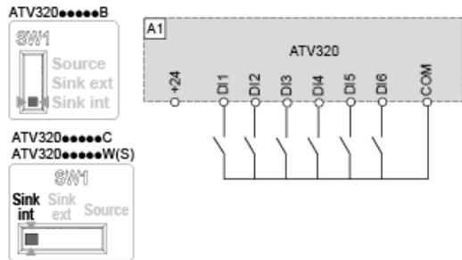
Switch SW1 set to "Sink Ext" position and use of an external power supply for the DIs.
