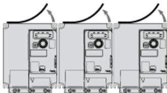
Mounting Type C: Individual, Ventilation Cover Removed
