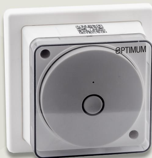
OP-SBWF01 IS A WiFi TIME SWITCH THAT WILL MOUNT ON A SINGLE PATTERNS. REMOTELY PROGRAMMABLE VIA THE USER'S HOME WiFi HUB AND A SMARTPHONE APP. VIA THE APP CAN BE PROGRAMMED FOR A TIMED SWITCHING SEQUENCE ON A 24 HOUR OR 7 DAY BASIS. CONTROLS A VOLT-FREE SWITCH WITH A RESISTIVE RATING OF 16 AMPERES.
