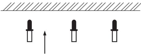
1. Drill 3 holes according the ceiling light installation hole, then put the plug in.
