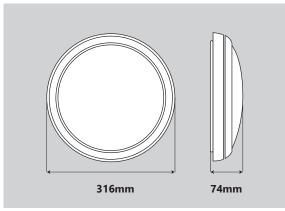
Detection Range: 10m(W) x 6m(H) Detection Angle: 30°~150°
